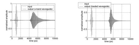
Figure 2: (a) Time domain representation of the pulse at the output of 84.6 cm length of hollow x-band waveguide, (b) and the loaded waveguide of the same length.
