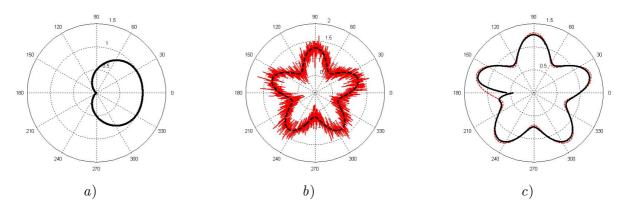
Figure : (a): function  $\widetilde{up}(\phi)$ , (b): radial signal without (dotted line) with noise (solid line), (c): filtered signal (solid line).
