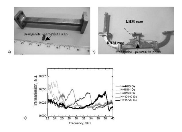
Figure : Photo of of the investigated metamaterial structures: (a) manganite-perovskite slab, (b) manganite-perovskite prism. (c)Transmission through manganite-perovskite metamaterial at various magnetic fields.
