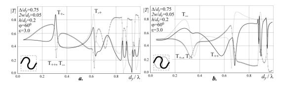
Figure : Normal incidence transmission of the DLS with identical gratings (a) and with reflection symmetric strips in adjacent gratings (b) The strips have the chiral shape.
