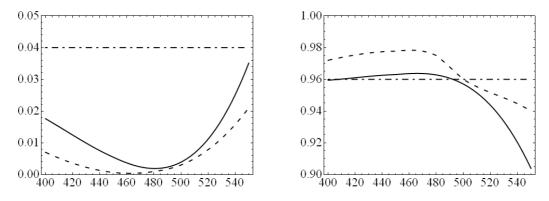
Figure: Reflection and transmittance spectra of composite material on glass substrate computed for normal incidence. Solid line corresponds to the case of three-layer antireflection structure. Dashed line is the case of optimized single-layer antireflection structure. Dot-dashed line corresponds to the case of the uncoated glass surface.
