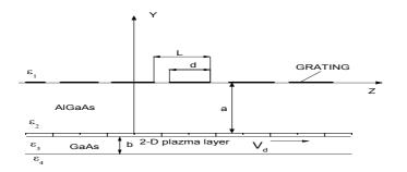
Figure : The electodynamic model under study.
