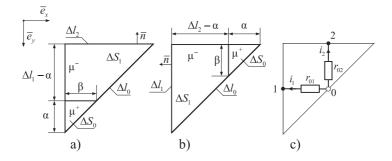
In the case shown on fig.1, a we have  $B_y = \text{const}$ ,  $H_x = \text{const}$  on  $\Delta S_1$ . By using  $\psi$ ,  $\bar{B} = [\text{grad}\psi, \bar{e}_z]$  we construct model of this element. The model is shown on fig.1, c, here
