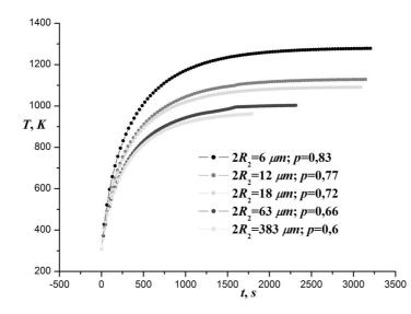
Fig.: Calculated heating curves of copper powder as a function of particle size.
