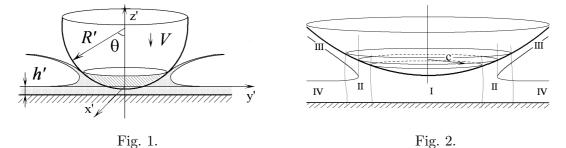
A main result of the analysis is that shallow-water impact is more dangerous than deep-water impact because stresses and the deformation of the shell increase as the thickness of the water layer decreases. But starting from some relatively large depth of the water, maximal values of the stresses and deflections remain constant with increasing water depth.
