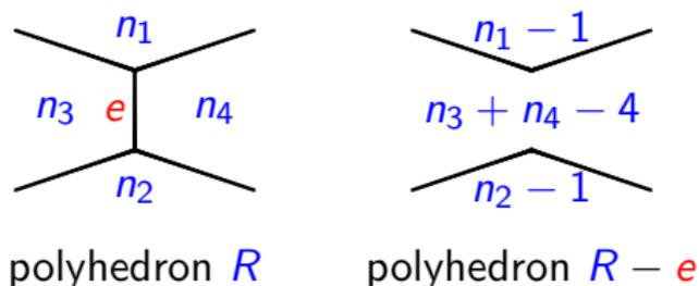
If  $R \in \mathcal{R}$  and  $e$  is such that faces  $F_1$  and  $F_2$  have at least 6 sides each and  $e$  is not a part of prismatic 5-circuit, then  $R - e \in \mathcal{R}$ .
