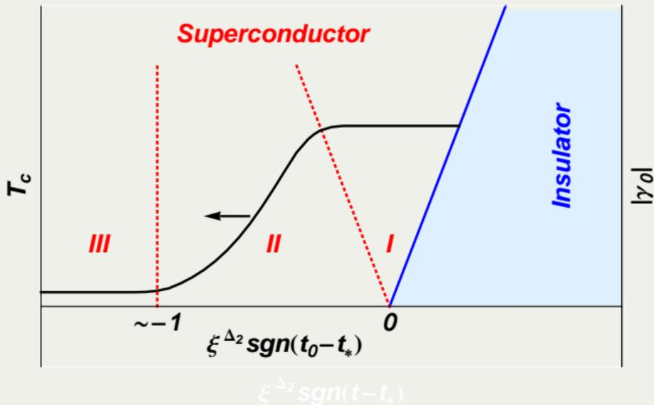
I:  $T_c = E_0 |\gamma_0|^{d/|\Delta_2|}$     II:  $T_c = \xi^{-d} E_0 \exp\left(-\frac{d}{a|\gamma_0|\xi^{|\Delta_2|}}\right)$     III:  $T_c = T_c^{BCS}$
