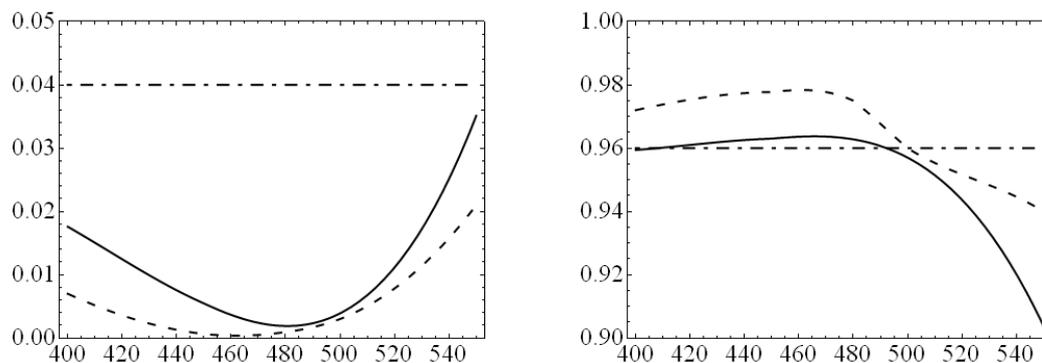
Figure: Reflection and transmittance spectra of composite material on glass substrate computed for normal incidence. Solid line corresponds to the case of three-layer antireflection structure. Dashed line is the case of optimized single-layer antireflection structure. Dot-dashed line corresponds to the case of the uncoated glass surface.
