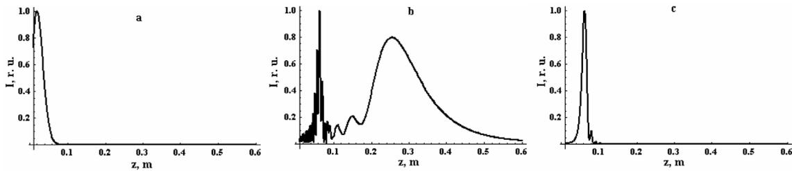
Figure : Normalized on its maxima paraxial intensity profiles of super short Bessel light beams formed by means of ideal (a), nonideal (b) conical lenses and axicon with photonic crystal on the cut apex (c).
