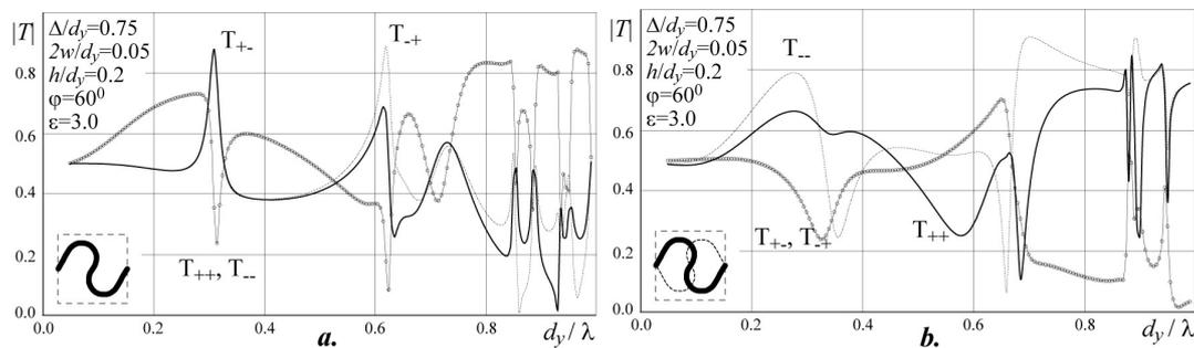
Figure : Normal incidence transmission of the DLS with identical gratings (a) and with reflection symmetric strips in adjacent gratings (b) The strips have the chiral shape.
