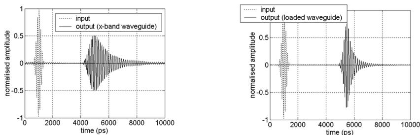
Figure 2: (a) Time domain representation of the pulse at the output of 84.6 cm length of hollow x-band waveguide, (b) and the loaded waveguide of the same length.
