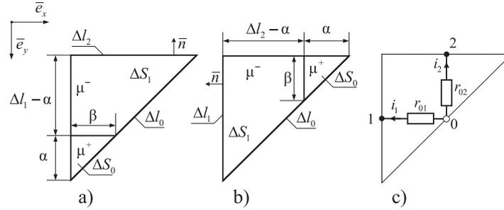
In the case shown on fig.1,a we have  $B_y = \text{const}$ ,  $H_x = \text{const}$  on  $\Delta S_1$ . By using  $\psi$ ,  $\vec{B} = [\text{grad}\psi, \vec{e}_z]$  we construct model of this element. The model is shown on fig.1,c, here
