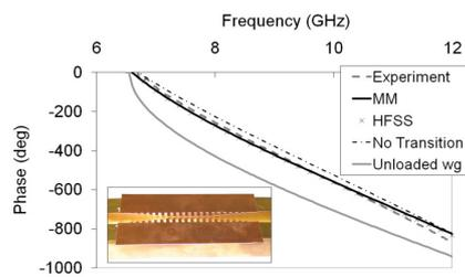
Figure 1: Fabricated prototype of a dispersion compensated waveguide: Measured and simulated unfolded transmission phase of S21 (unfolded phase for transmission along 78 mm of unloaded x-band waveguide shown for comparison).
