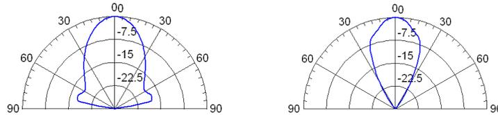
Figure 4: E-plane normalised radiation pattern for 2-layer antenna 6 at a) low-end bandwidth frequency 12.3GHz, b) upper-end bandwidth frequency 14.25GHz.
