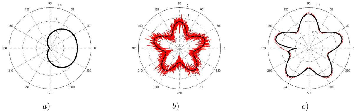
Figure : (a): function  $\widetilde{up}(\phi)$ , (b): radial signal without (dotted line) with noise (solid line), (c): filtered signal (solid line).
