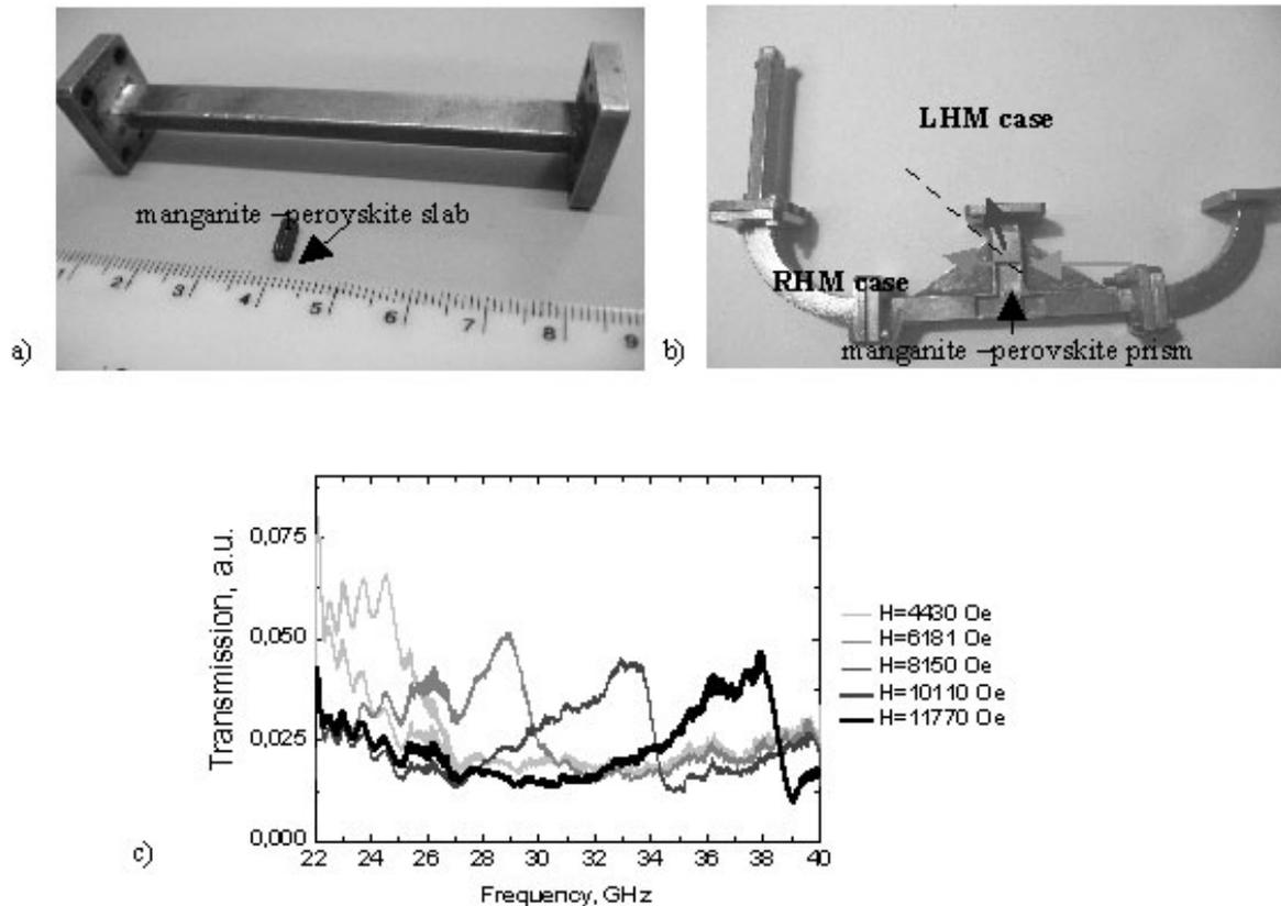
Figure : Photo of of the investigated metamaterial structures: (a) manganite-perovskite slab, (b) manganite-perovskite prism. (c) Transmission through manganite-perovskite metamaterial at various magnetic fields.
