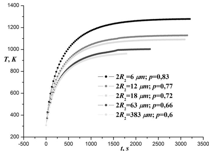
Fig.: Calculated heating curves of copper powder as a function of particle size.
