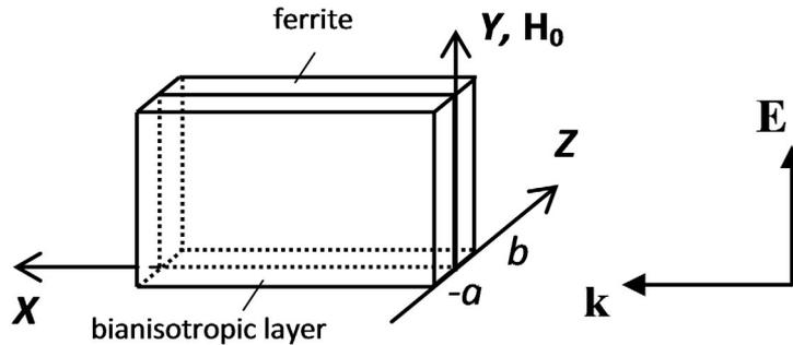
Figure : A bianisotropic-ferrite metasandwich in free space;  $\mathbf{k}$  and  $\mathbf{E}$  are the wave vector and electric field of an incident wave,  $\mathbf{H}_0$  is a magnetostatic field.
