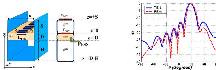
Figure 3: (a) 1D Fabry-Perot leaky-wave antenna formed by a parallel-plate waveguide loaded with a dipole-based FSS acting as a PRS and transverse equivalent network of the structure, (b) Radiation pattern of the designed PRS-LWA (LFSS=8mm,  $f=15\text{GHz}$ ).
