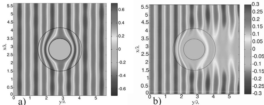
Fig. Magnetic field (Hz) amplitude distribution of the lossless (a) and a lossy (b) ideal cylindrical cloak.
