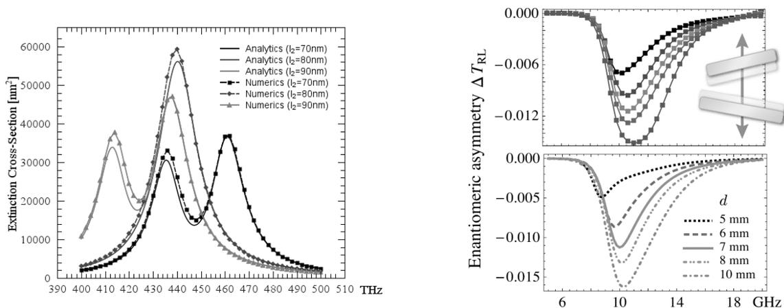
Figure: (Left) Gold nanorods dimer. Extinction cross-section of a pair of parallel gold nanorods of different length. One rod has fixed length  $l_1 = 80$  nm, distance between rods is  $d = 100$  nm. Com-
