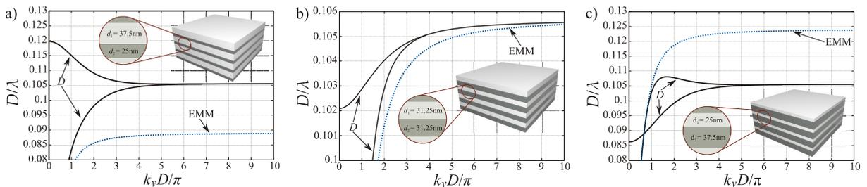
**Fig. 1.** The dispersion diagrams and geometry of the MDNs composed of alternating HfO<sub>2</sub> and Ag layers. The permittivity of HfO<sub>2</sub> is assumed to be equal to  $\varepsilon_1 = 4.6$ . The permittivity of silver is given by Drude model:  $\varepsilon_2 = 1 - \omega_p^2/\omega^2 = 1 - \lambda^2/\lambda_p^2$ , where  $\lambda_p = 2\pi c/\omega_p = 250$  nm. The ratio of layers thicknesses is varied as follows: a)  $d_1 = 1.5d_2$ , b)  $d_1 = d_2$ , and c)  $d_2 = 1.5d_1$ .
