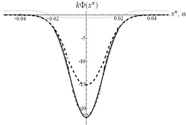
**Figure 1.** Behavior of the phase  $k\Phi(x^*) = k\Phi(x^*, x^*, 0, 0)$  for the case without treatment (dotted line), for  $D = D_0 = 28\text{cm}$  (dashed line), for  $D = D_0 = 35\text{cm}$ , (dash-dotted line) and for  $D = D_0 \sim Z$  (solid line).
