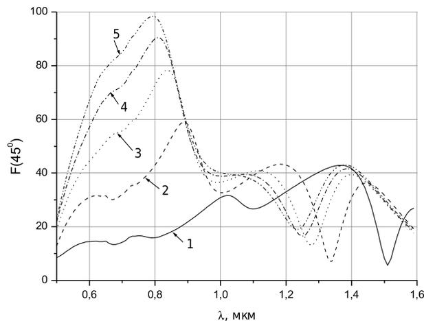
**Fig. 1.** Resonant characteristics of nanodipole. Material of dipole and substrate - ZnO,  $a=50\text{nm}$ ,  $L=1\mu\text{m}$ ; curves 1 to 5 designate thickness of metal cover 10, 20, 30, 40, 50 nm.
