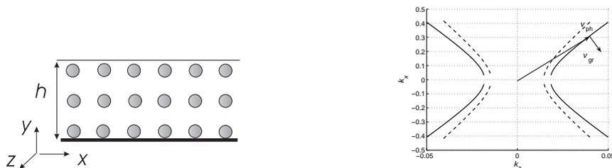
**Fig. 2.** Left: Cross-section of a planar waveguide consisting CNTs. Right: Isofrequencies, calculated at 10 THz (solid) and 8 THz (dashed line).
