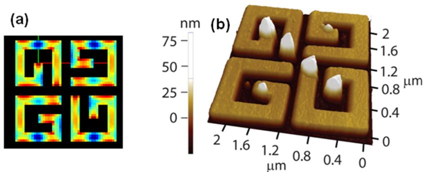
**Figure 1 | A high resolution imprint of the plasmon hotspots.** In (a), theoretical simulation of the electric currents in the nanostructures. In (b), after illumination of the sample, the localized field enhancements are imprinted on the nanostructures. Subsequently, an Atomic Force Microscopy image reveals the precise location of the hotspots.
