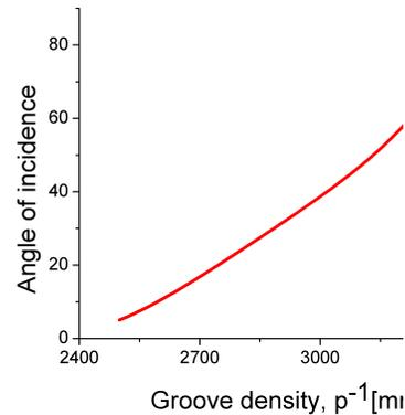
Fig. 2. The incidence angle as a function of the grating period for a fixed tilt angle  $\alpha = 62.7^\circ$ .
