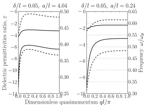
FIG. 2. Dispersion for 1st and 2nd Brillouin zones: solid lines correspond to FIG. 1a), dashed lines to FIG. 1b). We plot the curve in terms of frequency  $\omega$  (right plot);  $\omega_p$  is the plasma frequency.
