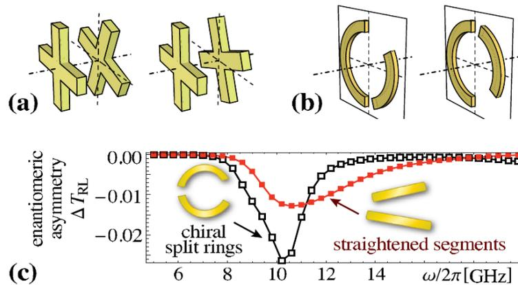
**Figure:** Example of (a) 3D and (b) 2D enantiomeric meta-atoms; (c) difference in transmission for left-handed vs. right-handed circularly polarized wave for split-ring vs. “straighened split-ring” (rod dimer) structure.
