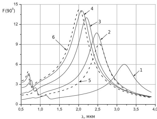
Fig. 1 Resonant characteristics of nanodipole made of ND made of ZnO (radius  $0.01 \mu\text{m}$ ,  $L=0.7 \mu\text{m}$ ) in case of different thickness copper layer. Copper layer 5, 10, 15, 20 nm – curves 1–4, accordingly. Curves 5, 6 – copper NV with radius 15 and 30 nm.
