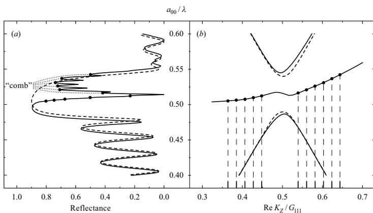
**Figure:** Calculated Bragg reflection spectra (a) and corresponding dispersion curves for the electromagnetic eigenmodes (b) of an opal-like photonic crystal film (assembled from polystyrene spheres of 300 nm in diameter) with the 20 monolayers thickness. The dashed curve describes the light diffraction from the only one system of crystal planes (111). The solid curve corresponds to the simultaneous diffraction from two systems of crystal planes (111) and  $(11\bar{1})$ .
