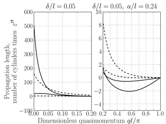
FIG. 3. Propagation length of surface plasmon mode times  $\text{Im } \varepsilon$ .
