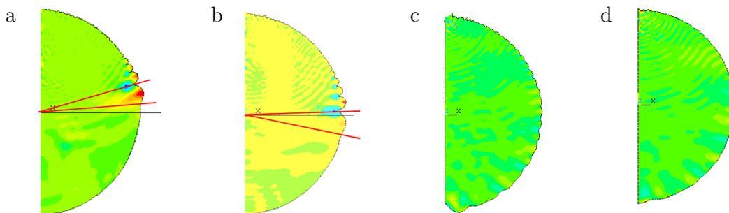
**Fig. 1.** Spatial-amplitude distributions of the global seismic field in the meridian section of the Earth: a –  $\rho = 3 \cdot 10^3 \text{ kg/m}^3$ ,  $\nu = 0.38$ , b –  $\rho = 2.1 \cdot 10^3 \text{ kg/m}^3$ ,  $\nu = 0.45$  (time delay after a shock  $\tau_1 = 2.5 \text{ ms}$ ), c – a shock on the free boundary, d – a shock on the crust-mantle interface ( $\tau_2 = 5.4 \text{ ms}$ ).
