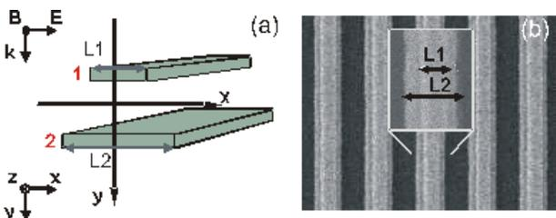
Fig. 1. (a) - Geometry of the double-wire structure considered in the theoretical model. (b) - SEM image of the experimental structure.
