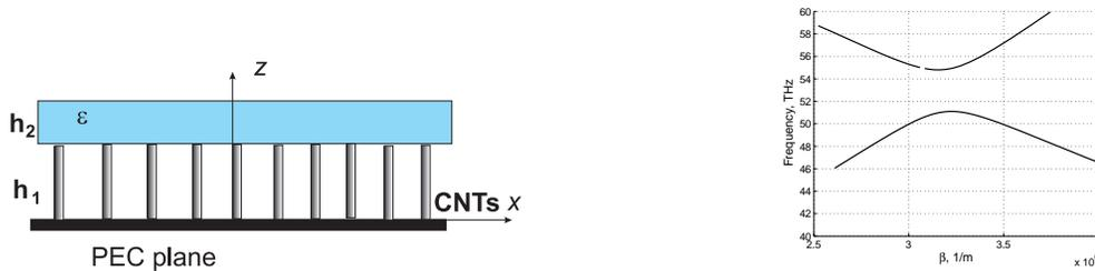
**Fig. 1.** Left: Schematic view of a vertically standing CNTs, adjusted to a dielectric slab. Right: Frequency versus the wave propagation constant  $\beta$ , calculated at  $h_1 = 1.2 \mu\text{m}$ ,  $h_2 = 1.5 \mu\text{m}$ .
