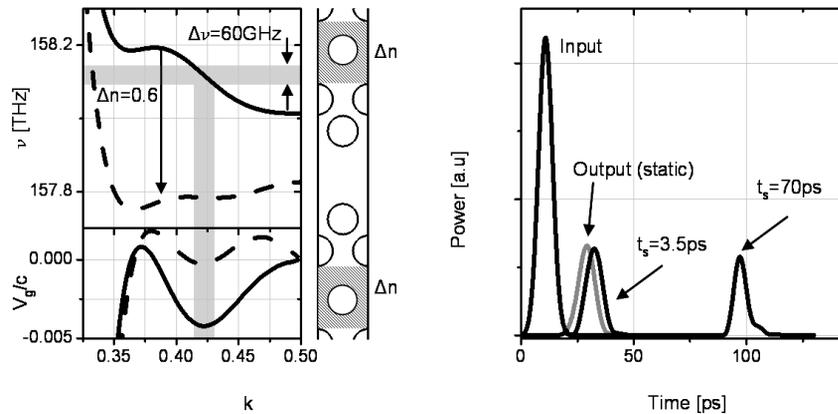
**Figure 1.** Left: Dispersion and group velocity of the guided mode in the initial state and after an applied refractive index change. The waveguide unit cell is also shown. Right: Numerical results for different storage times  $t_s$ .
