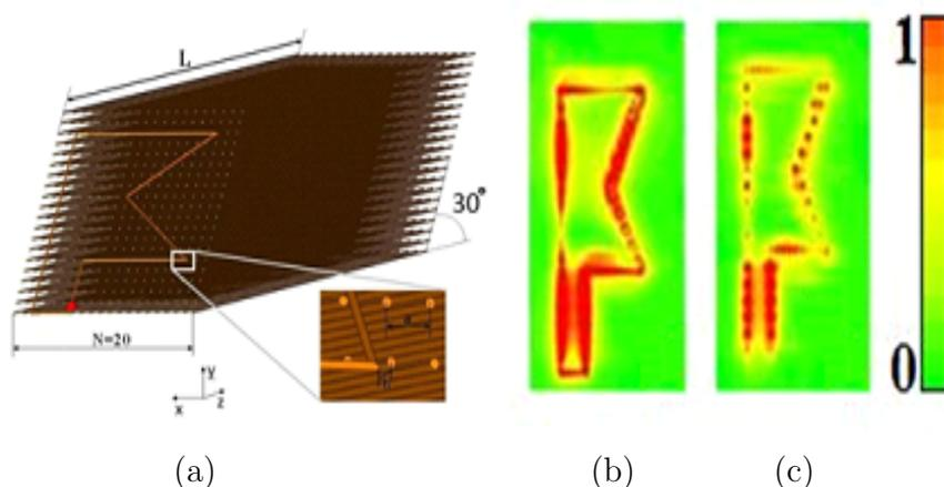
**Fig. 1.** a) Geometry of the sloped lens with “interface plane angle” = 30° formed by the wire medium and the source in the form of the flag. Distribution of  $E_y$  electric field component at the vicinity of the source <4 mm from the front lens interface> (b) and in the image plane <4 mm from the back lens interface> (c). The results are presented for the frequency of the first Fabry-Pero resonance (60MHz) normalized by the maximum value of electric field intensity.
