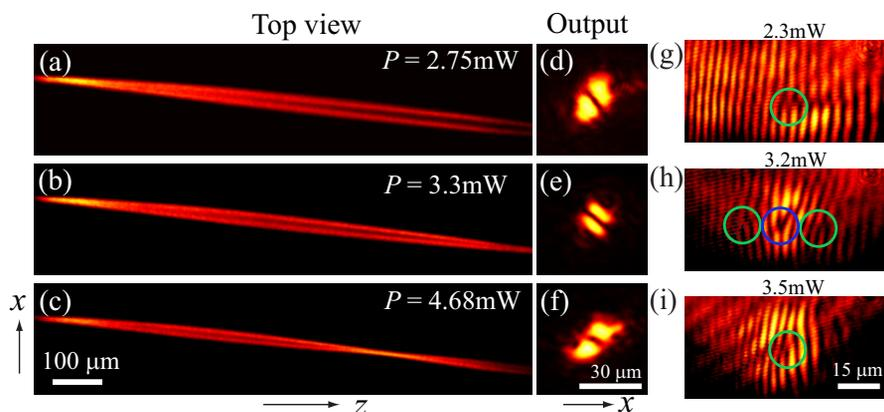
**Fig. 1.** Generation of a dipole azimuthon demonstrating the power-controlled twist and breathing of the beam. (g-i) Experimental interferograms with topological reactions of non-local dipole azimuthon. The circles indicate positions of phase singularities with charges +1 (green) and -1 (blue).
