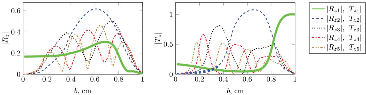
**Fig. 1:** Dependence of  $|R_z|$  (left) and  $|T_z|$  (right) on channel radius  $b$  in the case of incidence of the 1st propagating mode; dielectric permittivity is equal to 7, waveguide radius is 1 cm, the frequency is 13 GHz, phase velocity of initial mode is equal to  $2c$ . Thick line — propagating modes, thin line — evanescent modes.
