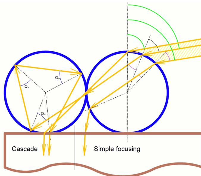
**Fig. 1:** Schematic view of mechanism of cascade focusing.
