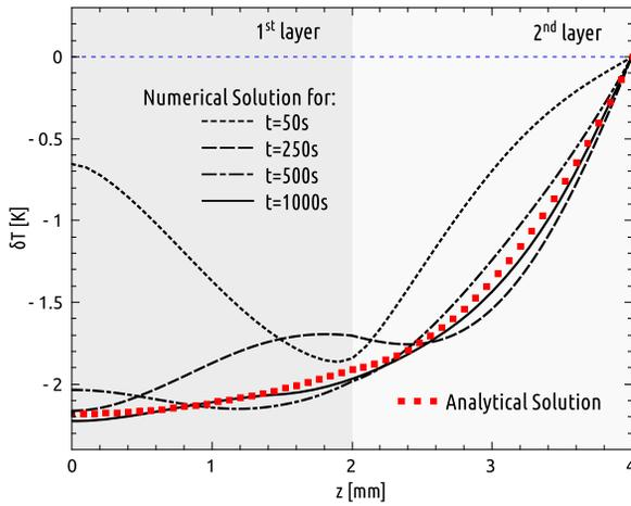
**Fig. 1:** The comparison of the analytical and numerical solutions of the heat conduction equation in the two-layered structure.
