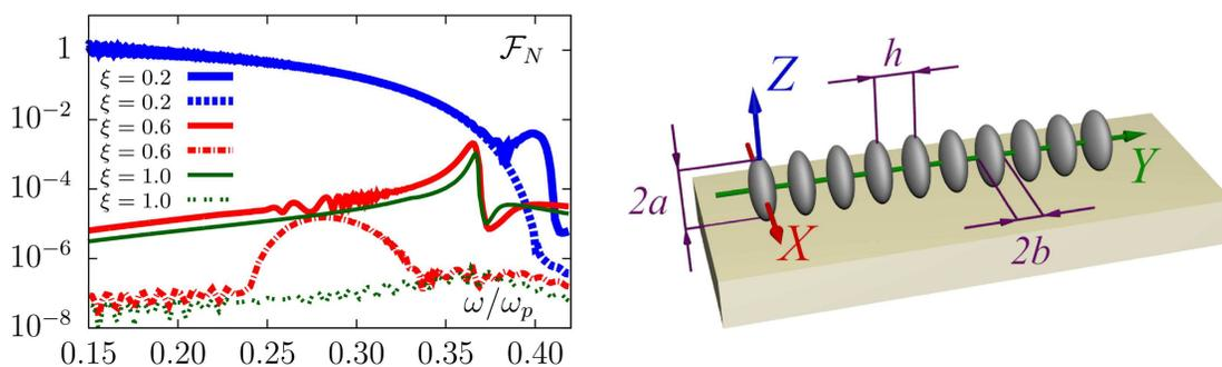
**Fig. 1:** Transmission spectra for chain consisting of  $N = 1001$  oblate nanospheroids located on a dielectric substrate (dot-dashed line) and in its absence (solid lines). The calculations were performed for polarization along  $X$  axis and for various values of the aspect ratio  $\xi = b/a$ . The shorter semi-axis is  $b = 8$  nm and the center-to-center interparticle distance is  $h = 24$  nm.
