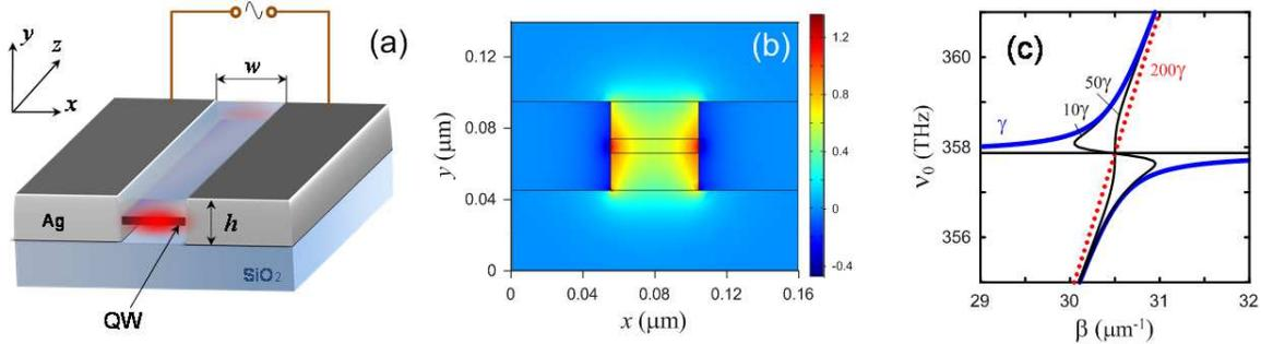
**Fig. 1:** (a) Schematic cross-section of the metallic slot waveguide configuration. QW denotes the quantum well embedded in the dielectric core (Al<sub>0.9</sub>Ga<sub>0.1</sub>As). (b) Poynting vector distribution is shown in the direction of plasmonic mode propagation at a frequency slightly below excitonic resonance. (c) Dispersion of the hybrid waveguide for different dephasing times of excitons. Real part of propagation vector.
