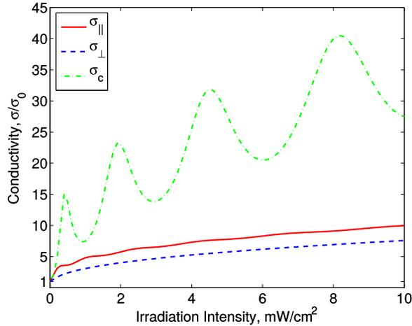
**Fig. 1:** The conductivity of 2DEG in a GaAs quantum well irradiated by a dressing electromagnetic field with the frequency  $\omega = 10^{11}$  rad/s at the temperature  $T = 0$  for  $\epsilon_F = 10$  meV.
