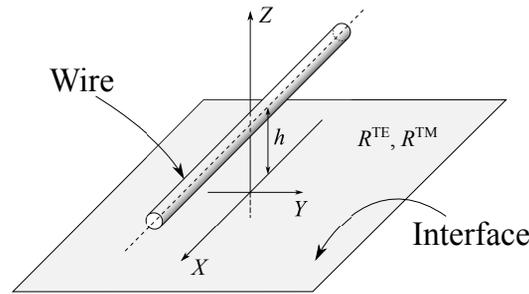
**Fig. 1:** Geometry of the problem: a section of an infinite thin wire over the interface at  $z = 0$ .
