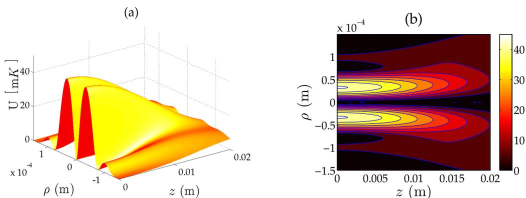
**Fig. 1:** (a) Dipole optical potential of a higher order Bessel–Gauss beam in function the transverse distance and the propagation distance. (b) Orthogonal projection.
