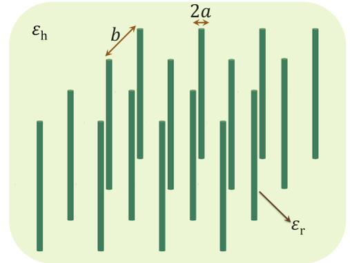
**Fig. 1:** Geometry of a square lattice wire medium.  $b$  and  $a$  are the lattice constant and the radius of the dielectric rod, respectively. In addition,  $\epsilon_h$  is the host medium permittivity and  $\epsilon_r$  represents the relative dielectric constant of the wire.
