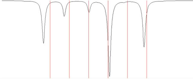
**Fig. 1:** Example of calculated hyperfine splitting line shape in the case of magnetic moment precession between easy magnetization axes.
