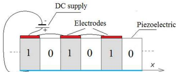
**Fig. 1:** Elastic, piezoelectric and permittivity properties of Area 0:  $C, e, \epsilon$ ; Area 1:  $C(E), e(E), \epsilon(E)$ .
