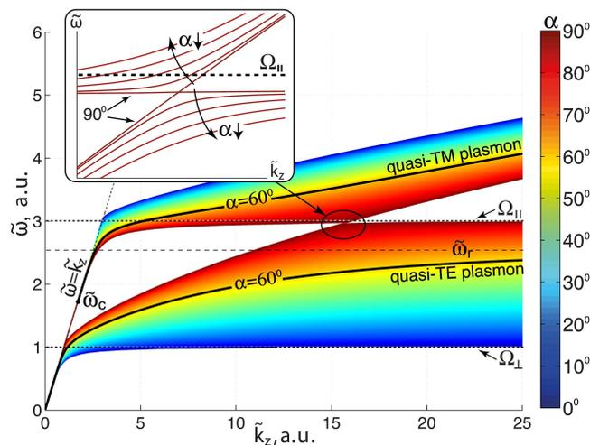
**Fig. 1:** Dispersion of wave vector  $\tilde{k}_z$  for the surface waves on hyperbolic metasurface for different propagation directions  $\alpha$ .
