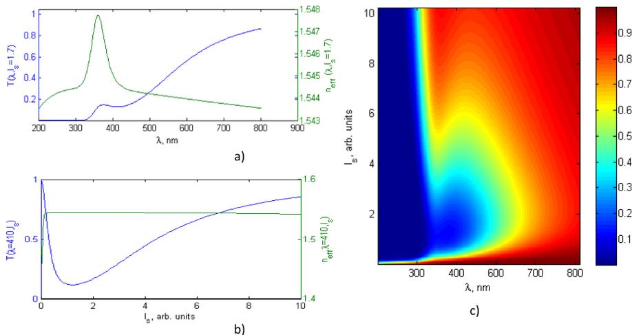
**Fig. 1:** Optical characteristics of the metamaterial:  $T$  and  $n_{eff}$  a) the wavelength dependence, b) dependence of external radiation, c) transmission spectrum  $T(\lambda, I_s)$ .
