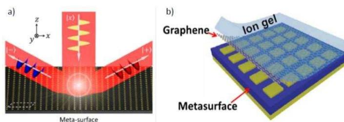
**Fig. 1:** a) Schematics of the 100%-efficiency photonic spin-hall effect realized at our reflective meta-surface, b) full-range phase modulator based on graphene metasurfaces.
