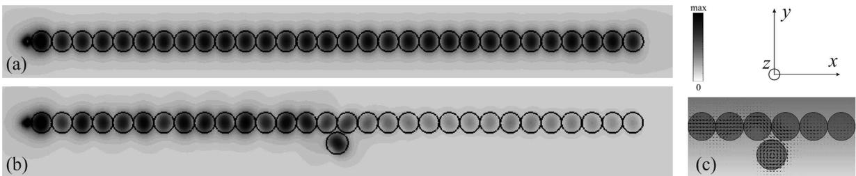
**Fig. 1:** Magnetic field distribution  $|\mathbf{H}|$  in (a) straight chain of dielectric particles and (b) chain with additional particle. (c) Power flow distribution in the center of the chain.
