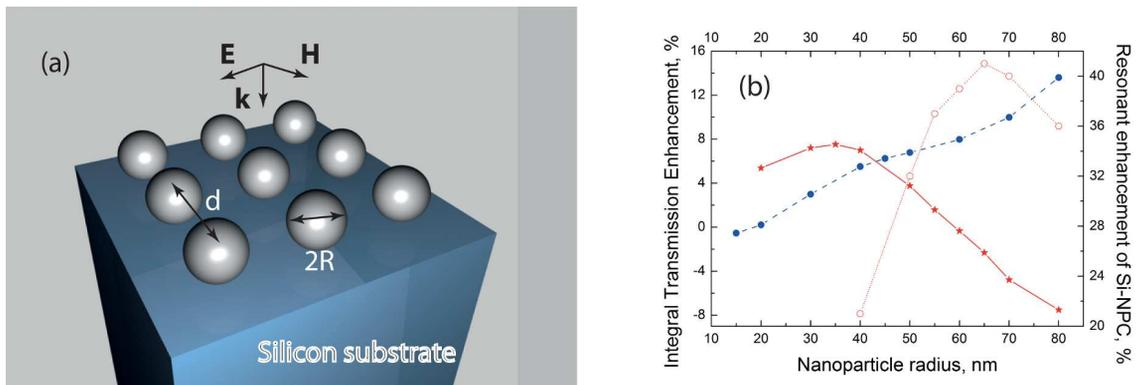
**Fig. 1:** (a) Square periodic array of spherical nanoparticles with radius  $R$  on the top of a-Si:H surface. (b) Left axes: integral enhancement for different type of coatings: Ag-NPC (blue circles) and Si-NPC (red stars). Right axes: the resonant enhancement for silicon coatings (red circles).
