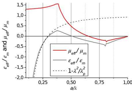
**Fig. 1:** Dependence of the effective permeability and permittivity of the structure on the ratio of the period ( $a$ ) to the wavelength ( $\lambda$ ),  $\lambda = 2\pi c/(\omega\sqrt{\varepsilon_m\mu_m})$ ,  $r = 0.05a$ . The conductivity of the wires over  $10^4$  S. Imaginary components of effective permeability and permittivity at these conditions are small.
