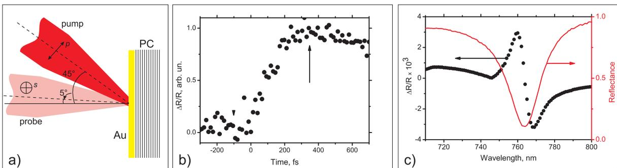
**Fig. 1:** (Color online) (a) Sketch of the experiment. (b) Transient reflectivity measured in the Au/PC sample at 760 nm. (c) Dots — experimental spectrum of the relative change in reflectivity of the Au/PC sample. Solid red curve — experimental reflectance spectrum of the Au/PC sample.
