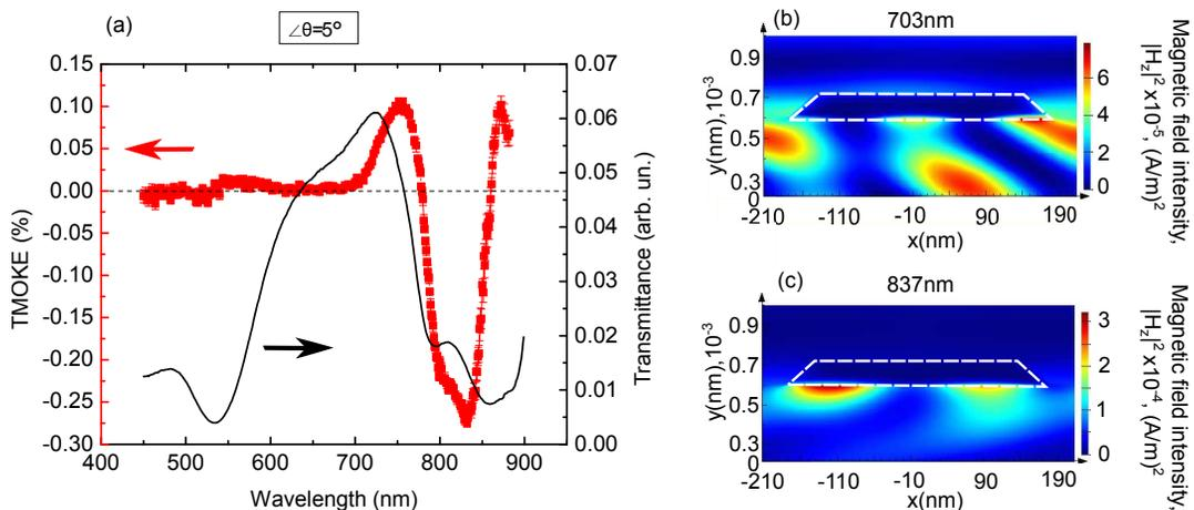
**Fig. 1:** a) Transmittance and the TMOKE spectrum of the magnetoplasmonic crystal. b,c) Numerical calculations of the intensity distribution of the magnetic field inside a strip of the magnetoplasmonic crystal for wavelengths 703 nm (+1st SPP mode) and 837 nm (-1st SPP mode). The white dashed curve is a strip profile. The incident angle of light is 5°.
