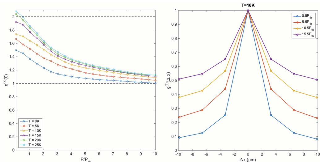
**Fig. 1:** a) Ground-state second-order temporal coherence function of the system of polaritons at zero delay as a function of the pump power for several temperatures. b) First-order spatial coherence as a function of the displacement from  $x = 0$  point at different pump powers.
