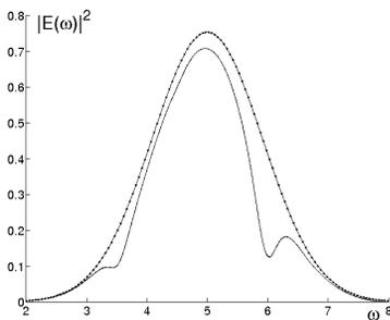
**Fig. 1:** Comparison of the original (asterisk line) spectrum and final spectra (solid line) in phase dependence studies.
