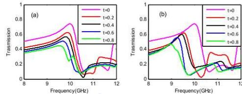
**Fig. 2:** Frequency response of the transmission for a) single-over-layer and b) double-over-layer for different over-layer thicknesses ( $t$ ).
