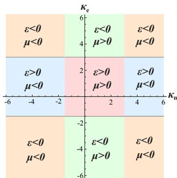
**Fig. 1:** Topological transitions in the structure composed of dielectric disks.  $\kappa_{e,m} = 4\pi\alpha_{e,m}/a^3$ ,  $\alpha_{e,m}$  is electric or magnetic polarizability of the disk.
