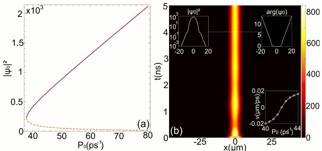
**Fig. 1:** (a) Bistability in the steady state: dependence of the exciton-polariton concentration,  $|\psi_0|^2$ , on the intensity of nonresonant pump,  $P_0$ , for the parameters:  $\gamma_0 = 0.025 \text{ ps}^{-1}$ ,  $R =$
