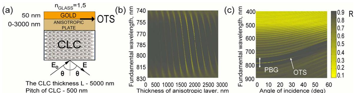
**Fig. 1:** a — The sketch of the studied CLC structure.  $E_0$  and  $E$  are the incident and reflected waves, respectively,  $\theta$  is angle of incidence. b — Reflectance spectrum of the modeled structure depending on the thickness of the anisotropic layer; c — Reflectance spectrum versus angle of incidence and wavelength of the radiation.
