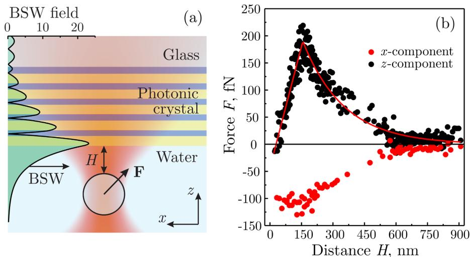
**Fig. 1:** (a) The experiment scheme. The calculated distribution of the incident BSW electric field amplitude is shown in green. (b) The  $x$ - (red dots) and  $z$ -coordinate (black dots) projection value of the measured force depending on the distance between the particle and the photonic crystal surface.
