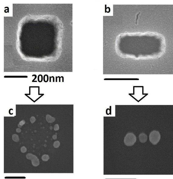
**Fig. 1:** SEM images of used electrodes: square (a), rectangle (b), and corresponding MIF-structures grown on the glass surface (c,d). Black scale bar below each figure corresponds to 200 nm.
