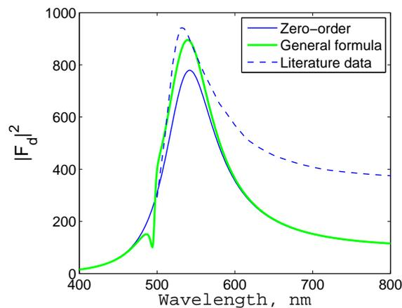
**Fig. 1:** Fluorescence spectrum of a quantum dot coupled to a golden nanosphere normalized to that of the single quantum dot. Thin line — zero-order model [1]. Dashed line — exact simulations of the semiclassical model (literature data). Thick line — our general formula.
