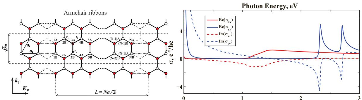
**Fig. 1:** Atomic structure (left column) and conductivity (right panel) of the array of armchair nanoribbons.
