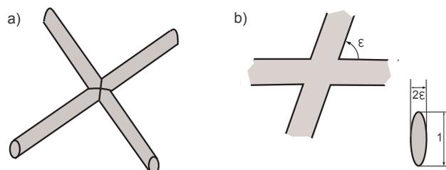
**Fig. 1:** The cruciform waveguide (a); nonorthogonal and elliptic cross section cases (b).
