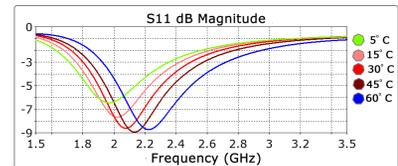
**Fig. 3:** Sensor application of the proposed MA with respect to temperature change.
