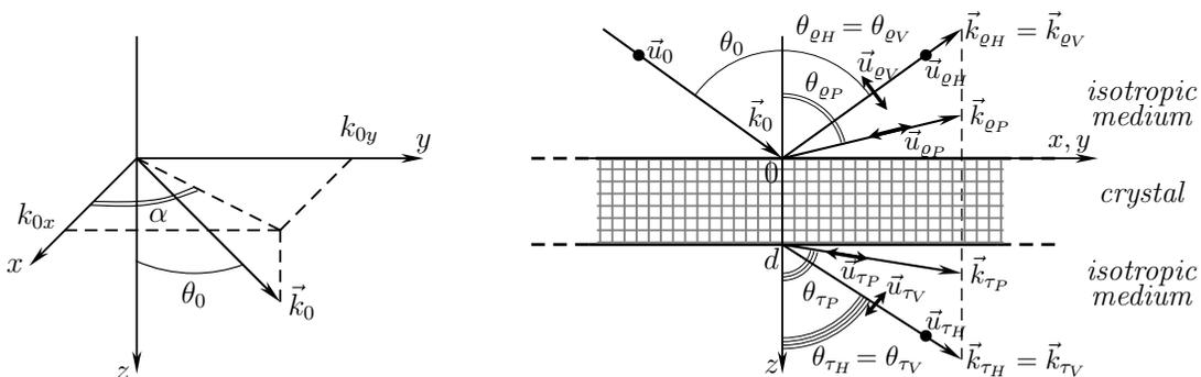
**Fig. 1:** The geometry of the *SH*-wave scattering
