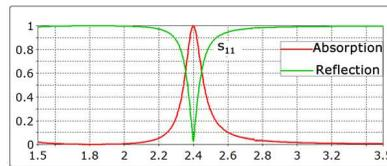
**Fig. 2:** Simulated reflection and absorption for the suggested MA.
