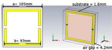
**Fig. 1:** Configuration and dimensions of the MA.
