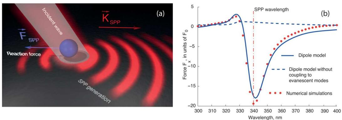
**Fig. 1:** (a) The geometry of nanoparticle attraction with SPP induced pulling force. (b) Spectral dependence of pulling force acting on a dielectric nanoparticle of radius  $R = 15 \text{ nm}$  placed above the silver substrate at the distance  $z = 27 \text{ nm}$ .  $F_0$  is the radiation pressure force in vacuum. Angle of incidence is  $35^\circ$ . The wavelength of SPP excitation is shown with dash-dot line.
