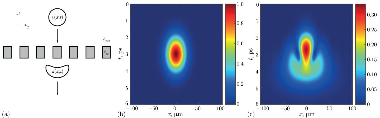
**Fig. 1:** (a) Pulse diffraction on resonant grating, (b) incident pulse envelope  $v(x, t)$ , (c) transmitted pulse envelope  $u(x, t)$ .
