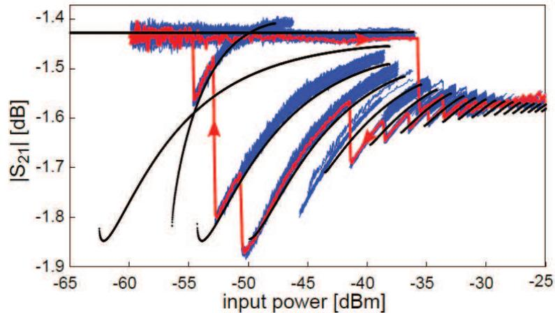
**Fig. 1:** Calculated (black) and measured (blue and red) transmission through the sample arrangement containing only a single SQUID. The red data show a hysteresis loop from low to high power and back. The red arrows indicate the direction of the sweep. The blue data are a collection of different power sweeps of varying length and initial conditions [1].
