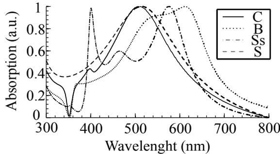
**Fig. 1:** Absorption of nanostructures for normal incidence (C — Conical, B — Barrel, Ss — Semi-sphere, and S — Sphere).
