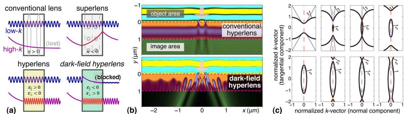
**Fig. 1:** (a) Illustration of metamaterial-based superresolution imaging approaches. (b) Comparison between the conventional [2] and dark-field [3] HL for externally illuminated dielectric nanospheres. (c) A variety of dispersion relations for periodic plasmonic multilayers [4].
