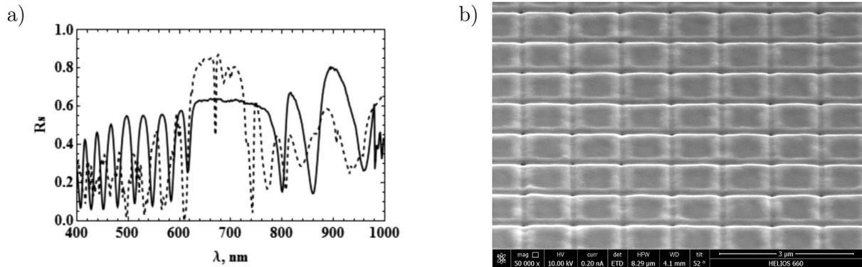
**Fig. 1:** (a) Reflection of a Bragg filter comprising 10 bilayers: angle of incidence  $\alpha = 45^\circ$ , thickness  $\text{SiO}_2$  layer  $h_1 = 135.35$  nm;  $\text{ZrO}_2$  layer  $h_2 = 96.68$  nm; thickness Al substrate  $h_3 = 150$  nm. The length and width of the cavities 300 nm and 100 nm correspondingly. Dashed line — computer simulation, solid line — experimental results. (b) REM picture of the surface of the multilayer.
