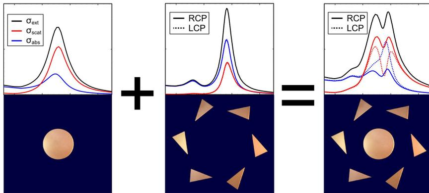
**Fig. 1:** Simulations of circular dichroism produced in the scattering and absorption losses of a planar chiral oligomer as a result of its Fano resonance.
