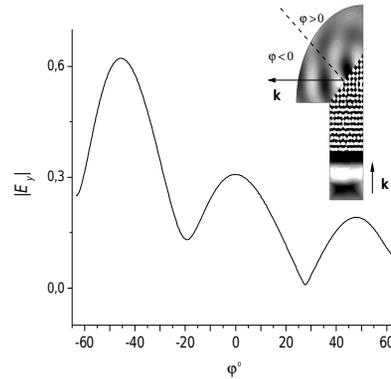
**Fig. 2:** The angular distribution of the absolute value of the vector of the field strength ( $E_y$ ) of the electromagnetic wave transmitted through the prism of the wired material. The dark area — the maximum values of  $E_y$ , light area — minimal.
