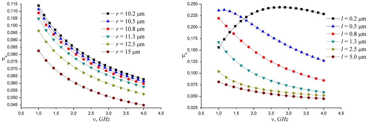
**Fig. 1:** Imaginary parts of the dynamic effective permeability of pure metallic conductive particles (left) and dielectric-coated conductor particles at different thickness of the conductive shell. The radius of the dielectric core is  $r = 10 \mu\text{m}$ . The conductivity is  $\sigma = 5.8e^7 \text{ S/m}$ .
