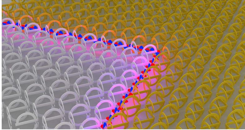
**Fig. 1:** Photonic topological insulator.
