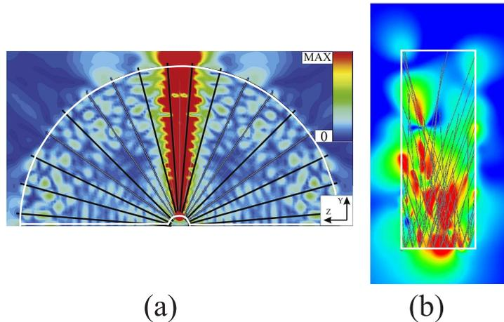
**Fig. 1:** Field distribution of hemispherical hyperlens (a) and randomized non-regular wire-medium (b) demonstrating the effect of radiating to free space energy from the poor radiating electrically small dipole. White line shows the contour of the structures.
