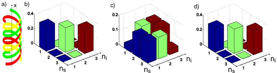
**Fig. 1:** (a) Scheme of coupled twisted waveguides. (b–d) Two-photon correlations ( $|\psi|^2$ ) between different waveguides at (b)  $z = 0$ , (c)  $z = L/2$ , (d)  $z = L$ .
