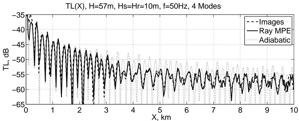
**Fig. 1:** The transmission losses for the cross-wedge sound propagation obtained by the three methods: source images, ray mode parabolic equation, adiabatic mode parabolic equation.
