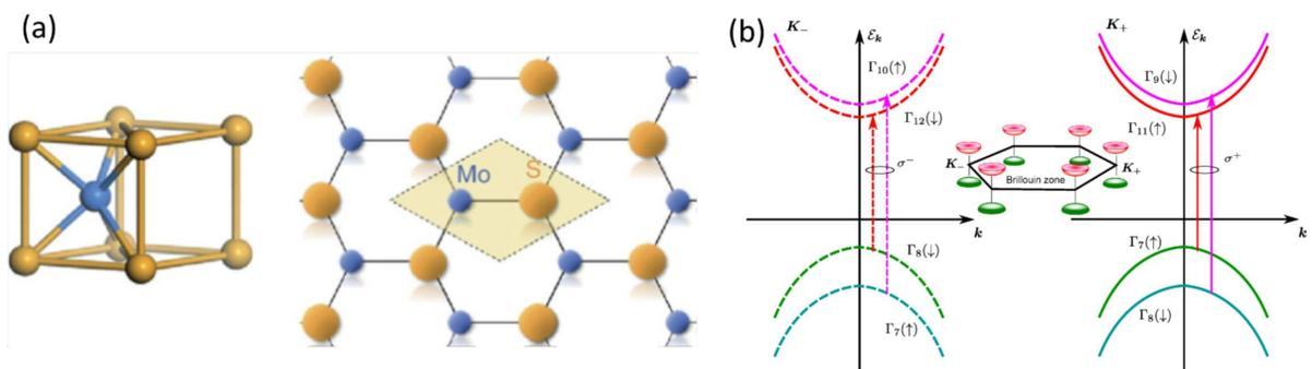
**Fig. 1:** (a) Schematics of the crystalline lattice of TMDCs on example of MoS<sub>2</sub>. (b) Sketch of the band structure and selection rules for the direct transitions in the vicinity of the  $\mathbf{K}_+$  and  $\mathbf{K}_-$  points.
