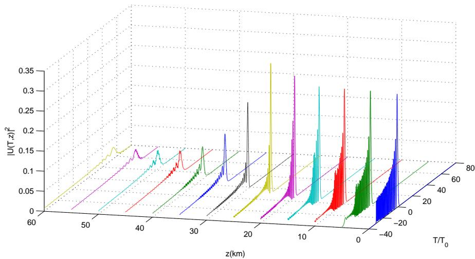
**Fig. 1:** Temporal evolution of time-truncated Ideal Airy pulse at different propagation distances
