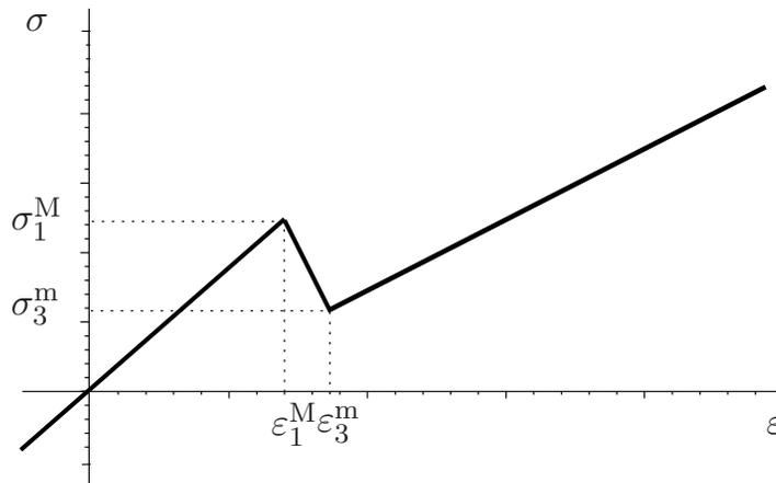
**Fig. 1:** The stress-strain curve for the material of a phase-transforming bar.
