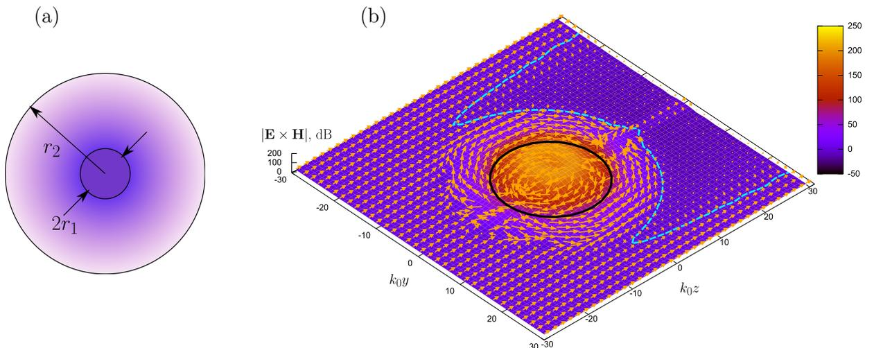
**Fig. 1:** (a) A spherical body with  $\varepsilon(r)/\varepsilon_0 = \mu(r)/\mu_0 = -r_2^2/r^2$ ,  $r_1 \leq r \leq r_2$ , and  $\varepsilon(r)/\mu(r) = \varepsilon_0/\mu_0$ ,  $\text{Im}[\varepsilon(r)] \rightarrow +\infty$ ,  $r < r_1$ . (b) Poynting vector plotted in the vicinity of a spherical body with structure shown in panel (a) which casts a shadow twice bigger than body's diameter.
