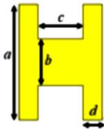
**Fig. 1:** Configuration fishnet-based-metamaterial with dimensions ( $a = 7.5$  mm,  $b = 4$  mm,  $c = 3$  mm, and  $d = 1.25$  mm).
