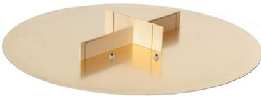
**Fig. 1:** Prototype top-side, including two monopoles for the 868 MHz and 2.4 GHz frequency band.
