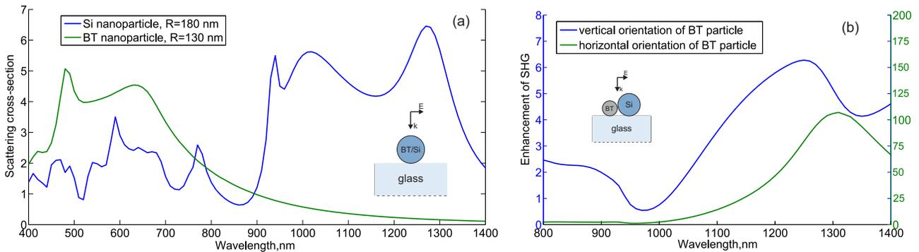
**Fig. 1:** (a) Elastic light scattering spectrum of a single BaTiO<sub>3</sub> nanoparticle (260 nm diameter) and single Si nanoparticle (360 nm diameter). The wavelength of the magnetic dipole resonance of the silicon nanoparticle is twice longer than for BaTiO<sub>3</sub> particle  $\lambda_{MD}^{Si} = 2\lambda_{MD}^{BaTiO_3}$ . (b) Enhancement of the second harmonic generation from BaTiO<sub>3</sub>-Si nanodimer comparing to a single BaTiO<sub>3</sub> particle.
