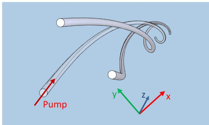
**Fig. 1:** Scheme of twisted circular array of coupled waveguides. Pairs of signal and idler photons are generated through spontaneous four-wave mixing from the pump.
