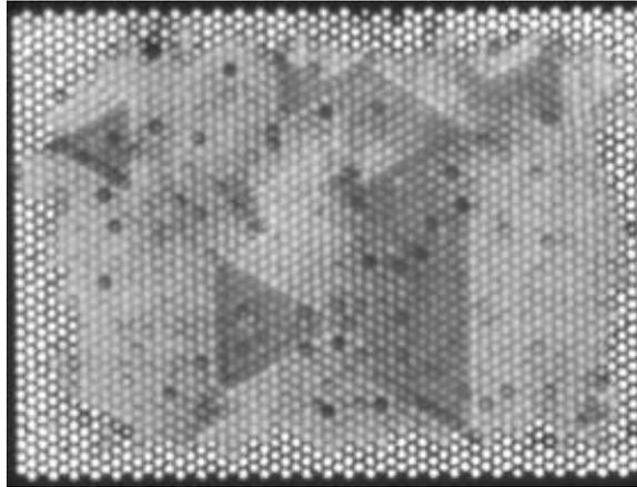
**Fig. 2:** Image of the metasurface in transmitted laser light (405 nm). The transmittance measurements and imaging were made using LSM710 (Zeiss) laser scanning.
