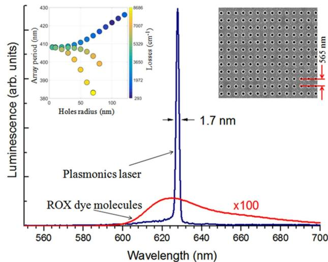
**Fig. 1:** Emission spectrum of plasmonic nanolaser radiated perpendicular to the surface of SPP crystal: above threshold (blue line), below threshold (red line). Inserts: (Right) SEM image of the plasmonic crystal; (Left) plasmonic crystal losses for bright and dark plasmonic modes.
