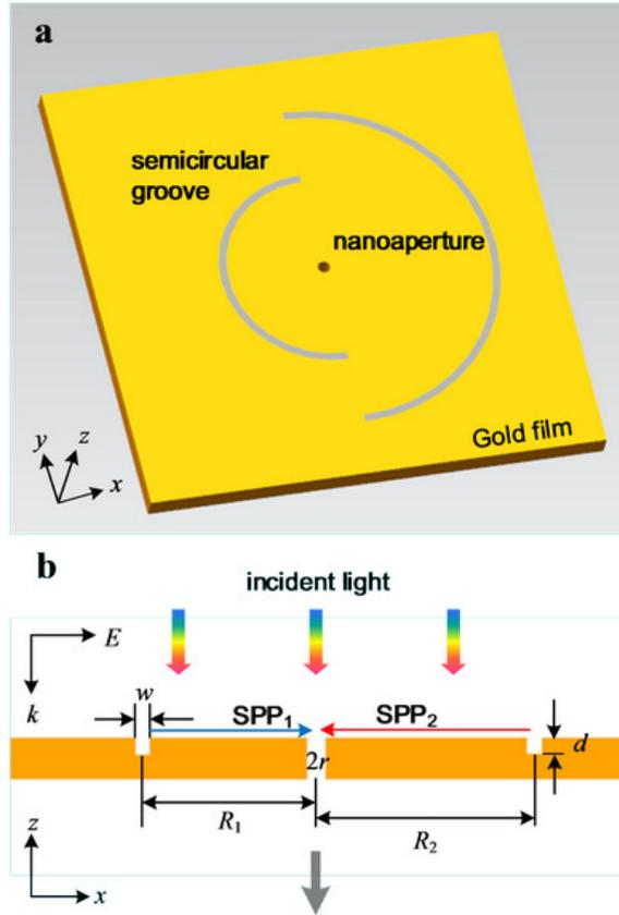
**Fig. 1:** a) Schematic of the proposed plasmonic interferometer. b) Side view and the working principle of the interferometer structure.
