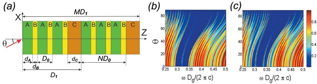
**Fig. 1:** Schematic of the bi-periodic 1D PC (a). Transmittivity of TE-mode as function of the normalized frequency  $\omega D_0/(2\pi c)$  and  $\theta$  for  $[(A/B)^{10}C]^2$  with  $d_A = 0.281 \mu\text{m}$ ,  $d_B = 0.341 \mu\text{m}$  and  $d_C = 0.796 \mu\text{m}$  (b), and  $d_C = 1.592 \mu\text{m}$  (c).
