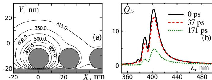
**Fig. 1:** The temperature  $T$  distribution at  $t = 1$  ns for first three OPW Ag NPs. Wavelength  $\lambda = 402$  nm and polarization along the  $X$  axis — (a). Transmission spectra of the OPW at different moments of time: the initial moment of time (solid line); the beginning of first NP melting (dashed line); the end of first NP melting (dotted line) — (b).
