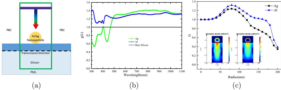
**Fig. 1:** Schematic diagram of simulation setup — (a), absorption enhancement vs wavelength for 100 nm diameter of different materials silver (Ag) and aluminium (Al) — (b), enhancement factor vs diameter for the same materials and absorption distribution in silicon (inset) — (c).
