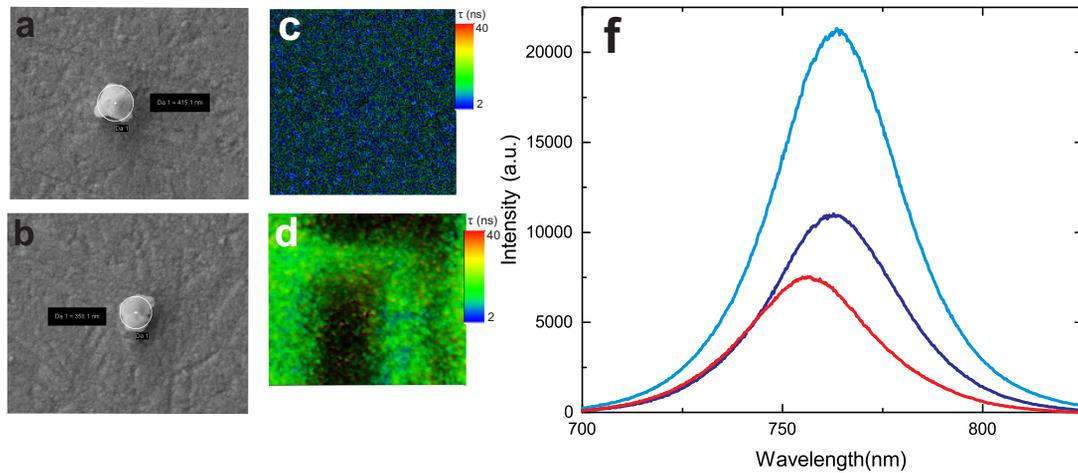
**Fig. 1:** SEM image (a,b) of resonant perovskite nanoparticles. Maps of average lifetime surface “old” perovskite sample (c) and perovskite nanoparticles on gold film surface (d). Photoluminescence spectra from different diameter perovskite nanoparticles.
