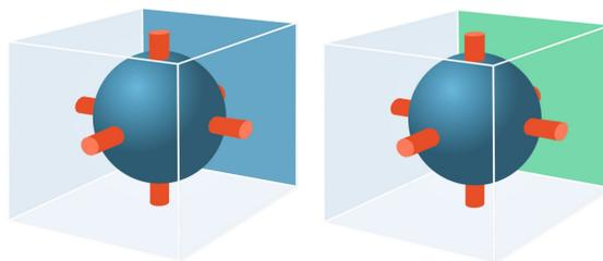
**Fig. 1:** The dual model of unit cell of spherical conductive particles connected to each other by conductive cylindrical bridges of radius  $r$ .
