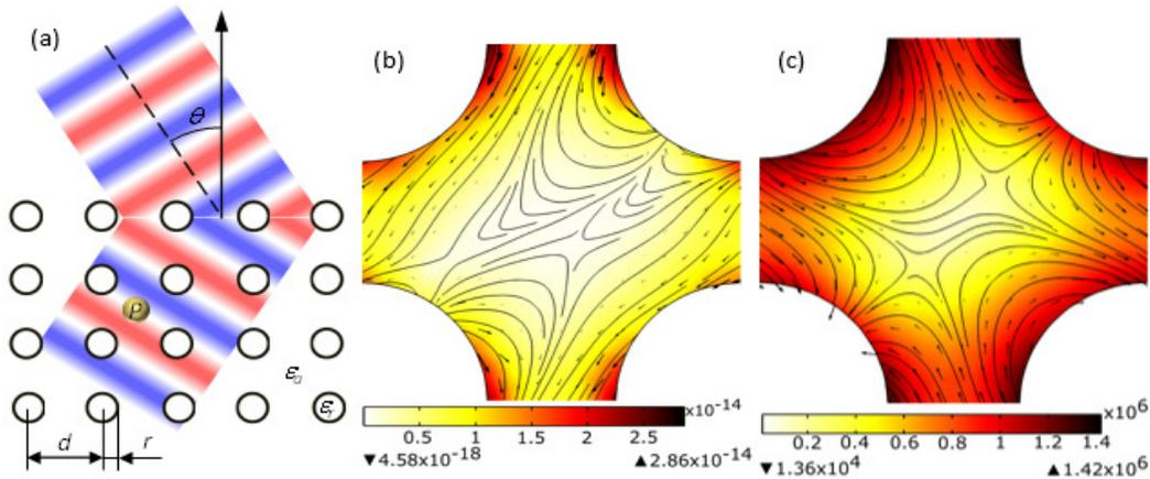
**Fig. 1:** (a) A left-handed photonic crystal with incident electric field  $\theta$  creates a negatively-refracting field. The particle P is modeled as a dipolar particle. (b) The forces within a unit cell of a left-handed photonic crystal is shown using the streamlines and arrowfield; the magnitude is shown using the color map. (c) The powerflow within the same unit cell as in 1b. is shown using lines and arrows; the color map indicates the norm of the electric field.
