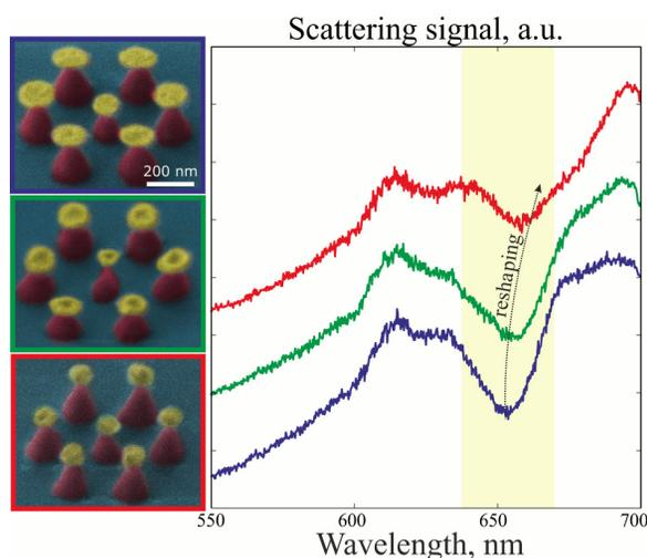
**Fig. 1:** Dark-field spectroscopy signals of the hybrid oligomer with gold nanodisks (blue curve), nanocups (green curve) and nanospheres (red curve).
