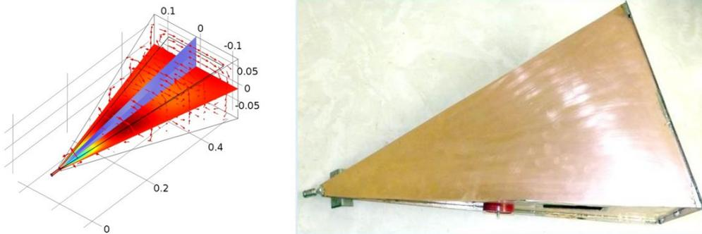
**Fig. 1:** Numerical model of GTEM-cell and its prototype.
