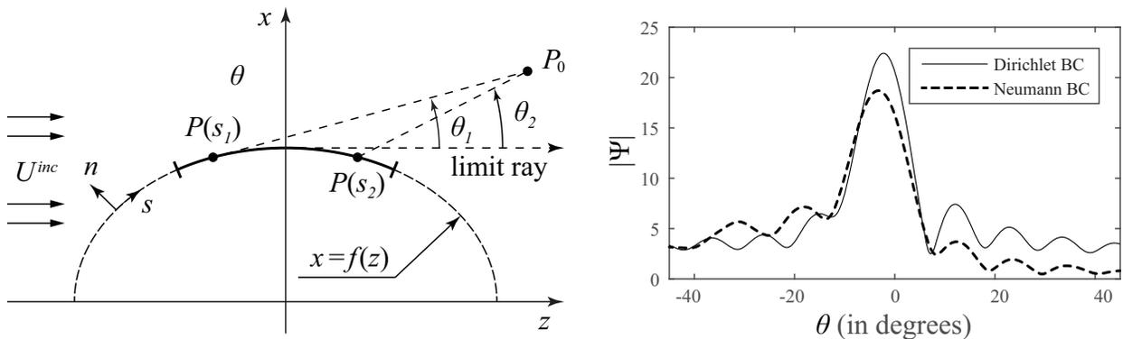
**Fig. 1:** Geometry of the problem (left); one from the numerical results for the modules of scattering amplitudes  $\Psi(\theta)$  (right).
