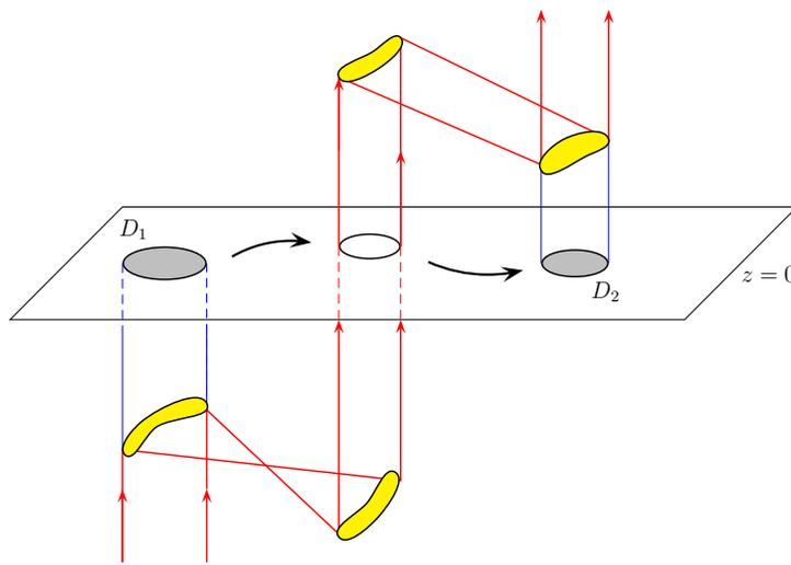
**Fig. 1:** A 4-mirror transformation of parallel bundles of rays induces a map from  $D_1$  to  $D_2$ .
