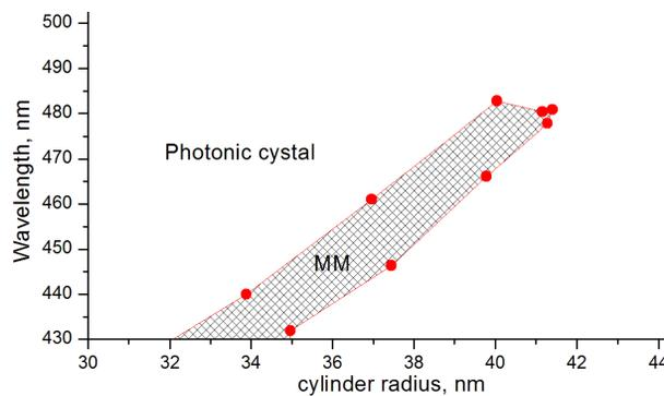
**Fig. 1:** The phase diagram of structure composed from the square lattice of silicon nanorods. The white area corresponds to photon crystal regime and the shaded area corresponds to metamaterial regime.
