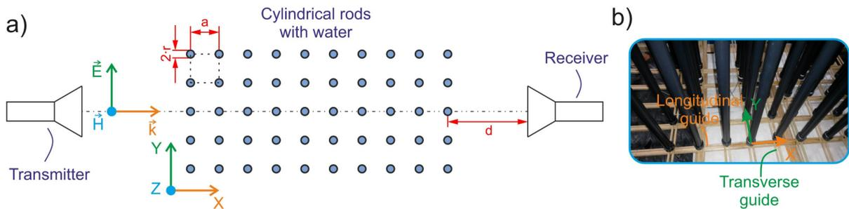
**Fig. 1:** (a) Schematic of the experimental setup. We arrange 5 by 10 rods in a square lattice placing the structure between a pair of horn antennas. (b) Photo of the experimental structure composed of a lattice of cylinders filled with water.
