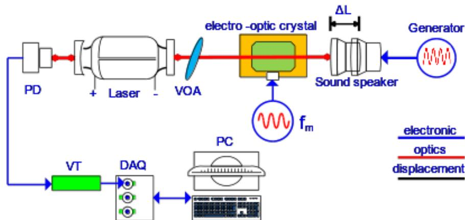
**Fig. 1:** The straightforward optical configuration of non-contact sound vibration measurement by phase-shifting self-mixing interferometer established on a dual-output He-Ne laser and an electro-optic modulator. VT denotes an adjustable resistor for photo current-to-voltage conversion, PC denotes computer for signal processing. DAQ denotes the analog-to-digital card. PD denotes a photo electric detector. VOA denotes the variable optical attenuator.
