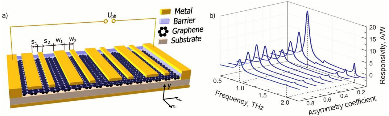
**Fig. 1:** (a) Schematic view of the DGG graphene structure; (b) Current responsivity vs. frequency and asymmetry coefficient  $s_1/s_2$ . Parameters of the calculations are  $w_1 = 1 \mu\text{m}$ ,  $w_2 = 0.25 \mu\text{m}$ ,  $s_1 + s_2 = 0.375 \mu\text{m}$ , and  $\gamma = 5 \cdot 10^{12} \text{ s}^{-1}$ .
