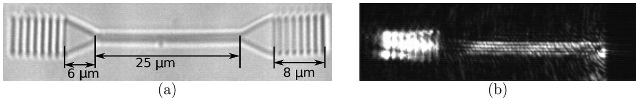
**Fig. 1:** a) Waveguide image obtained by optical microscopy. b) Waveguide image via leakage radiation microscopy. Light coupled through right grating, which were shut to prevent overexposure of a camera.
