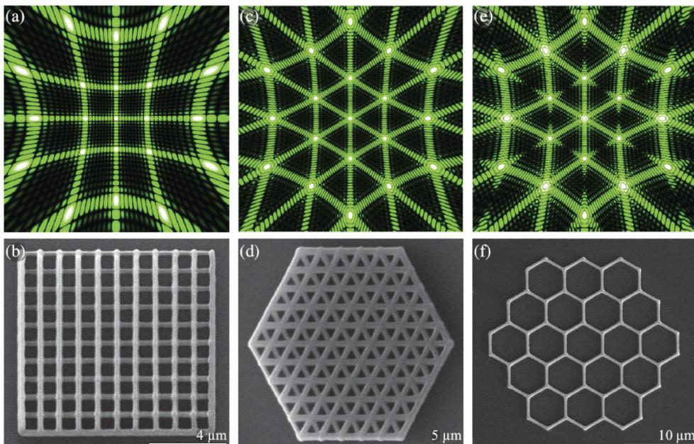
**Fig. 1:** Calculated diffraction patterns for square (a), triangular (c) and graphene (e) photonic structures on a flat screen positioned behind the sample. SEM images of the square (b), triangular (d) and graphene (f) photonic structures fabricated by the two-photon polymerization method.
