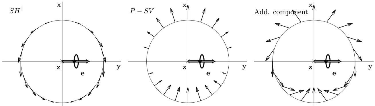
**Fig. 1:** Reflected wavefield components polarization patterns for a source with  $\mathbf{e}$  torque.
