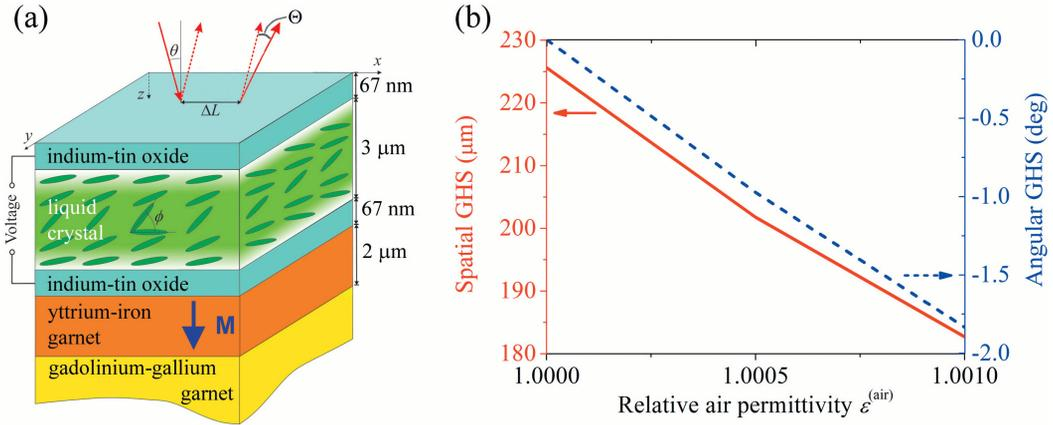
**Fig. 1:** (a) Schematic of the structure.  $\theta$  is the incidence angle,  $\phi$  is the tilt angle of the LC molecules,  $\mathbf{M}$  is the saturation magnetization in magnetic film. The spatial and angular GHSs are  $\Delta L$  and  $\Theta$ . (b) Variation of the GHSs for  $\varepsilon^{(\text{air})}$  varying from 1.000 to 1.001.
