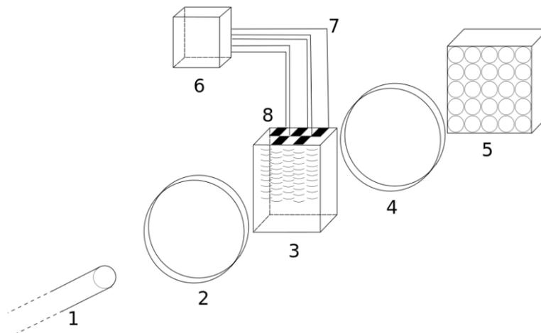
**Fig. 1:** Scheme of  $1 \times N$  commutator based on multichannel acousto-optic deflector: 1 – optical fiber; 2, 4 – lenses; 3 – acousto-optic cell, 5 – set of output optical fibers; 6 – amplifier; 7 – service power supply; 8 – multi-sectional piezoelectric transducer.
