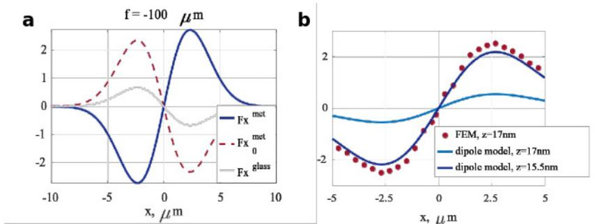
**Fig. 1:** Optical anti-trapping of a bead in Gaussian beam of waist  $10 \mu\text{m}$  focused below ( $f = -100 \mu\text{m}$ ) the air-silver interface. Dielectric particle of radius  $R = 15 \text{ nm}$  and dielectric permittivity  $\epsilon = 3$  is lying on metal ( $z = 15 \text{ nm}$ ). The wavelength  $\lambda = 342 \text{ nm}$  corresponds to resonance of surface plasmon.
