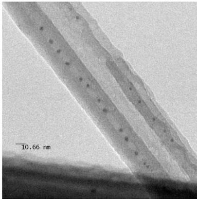
Figure shows nanotubes of chrysotile with gold as imaged in a JEM-2100F transmission electron microscope. As can be seen, the chrysotile nanotubes are filled with gold nanoclusters, whose diameter is less than 5 nm. They are located approximately at the same distance.
