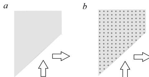
**Fig. 1:** Reflection coefficient measurement. a) Dielectric, b) Wire medium.
