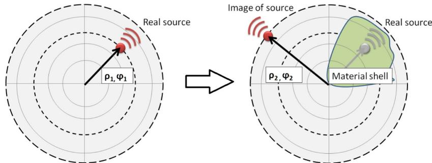
**Fig. 1:** Principle of transformation with virtual delocalization of emission source at the another radial and angular position.
