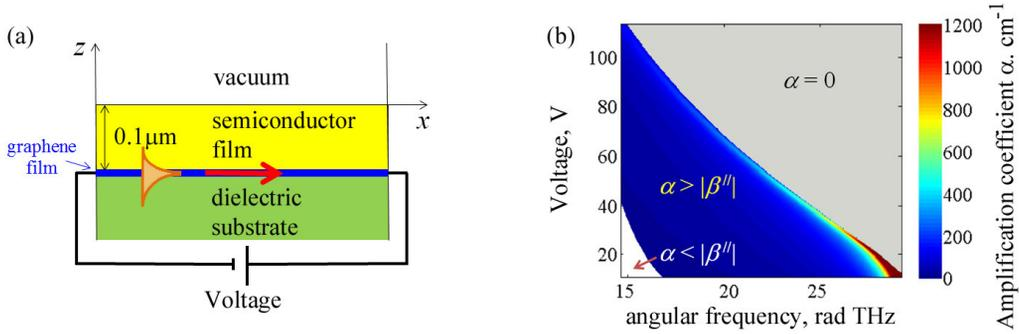
**Fig. 1:** (a) Schematic of the structure: a semiconductor film with deposited graphene is placed between semi-infinite dielectric substrate and vacuum. The arrow shows the directions of SSP wave propagation and electrons flux in graphene under an applied voltage. (b) Amplification coefficient  $\alpha > |\beta''|$  of SPP as function of the wave angular frequency and applied voltage. The grey and white areas correspond to  $\alpha = 0$  and  $\alpha < |\beta''|$ , respectively.
