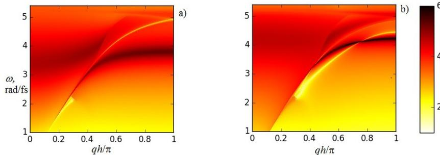
**Fig. 1:** Dispersion properties for various components of polarization of wave that propagate in a chain of nanoparticles that locate on the Silver substrate in the environment of silicon dioxide.
