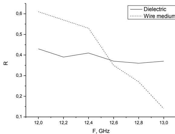
**Fig. 2:** Frequency dependencies of the coefficient of reflection of wire material and dielectric, angle of  $45^\circ$
