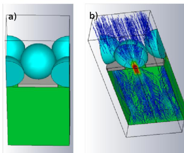
**Fig. 1:** (a) A unit cell of the structure and (b) Pointing vector in the case of forward transmission [2].
