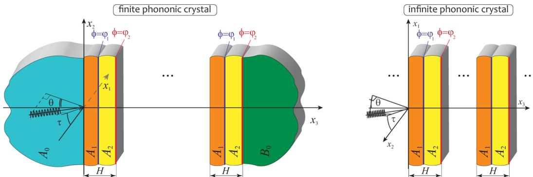
**Fig. 1:** Layered piezoelectric phononic crystal with electroded interfaces.
