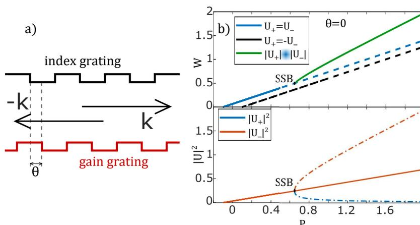
**Fig. 1:** a) Schematic view of a waveguide with periodical index and gain gratings. b) Bifurcation diagram for spatially uniform states. Upper panel shows dependence of the full field intensity of states on gain  $W = |U_b|^2 + |U_d|^2 = |U_+|^2 + |U_-|^2$ ; dashed lines indicate dynamically unstable states. Lower panels demonstrate intensities of counter-propagating waves; by solid and dash-dotted different branches from corresponding upper panel are shown.
