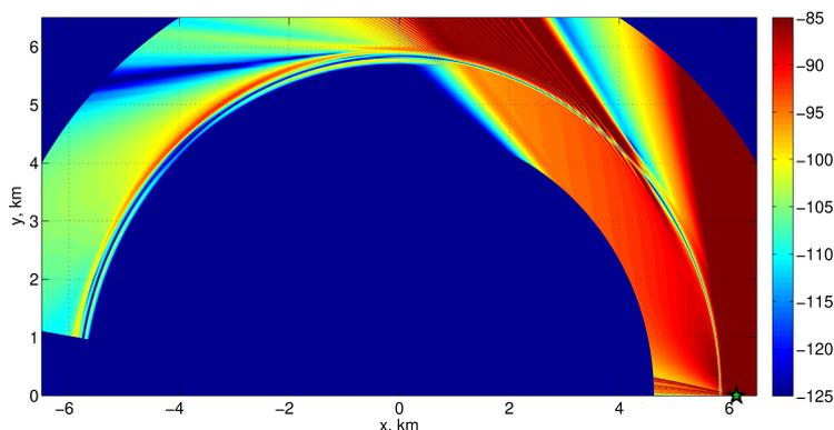
**Fig. 1:** Contour plot of the magnitude of acoustic field as a function of horizontal coordinates  $x, y$  (in dB re 1 m) at the depth  $z = 10$  m due to a point source in a shallow sea. Water depth decreases between the isobaths  $r = 5.8$  km and  $r = 6$  km from 26 to 24 m. Source position is marked by a star.
