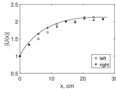
**Fig. 1:** Comparison between theoretical value of total field on the cone surface calculated from [1] and field measured in the diffraction experiment.
