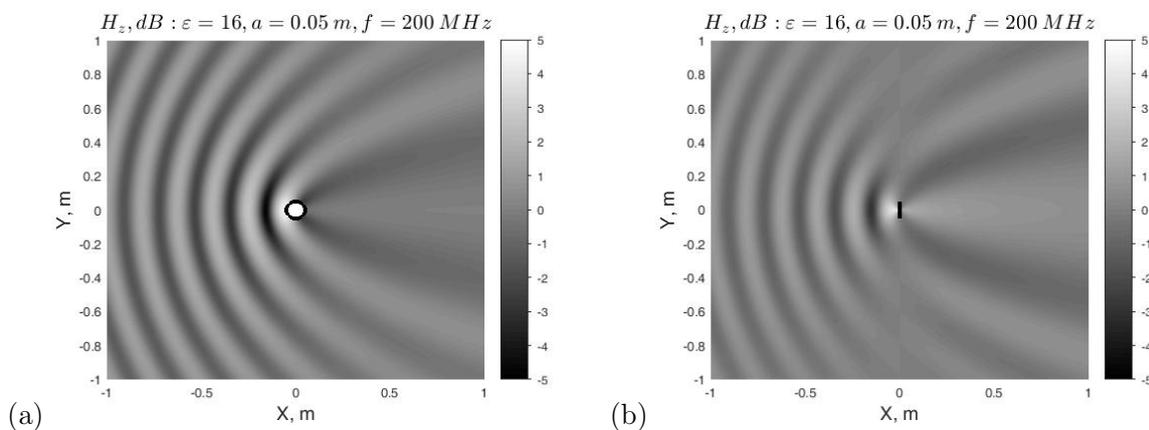
**Fig. 1:** Scattered field amplitude distribution for two diffracting objects: a) cylinder, b) plane strip.
