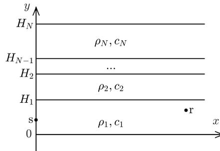
**Fig. 1:** Multilayered waveguide.
