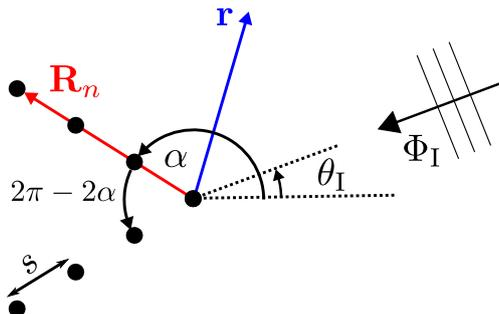
**Fig. 1:** Diagram of the point scatterer wedge with scatterers located at  $\mathbf{R}_n$ , the position vector  $\mathbf{r}$  and the incident wave  $\Phi_I$ .
