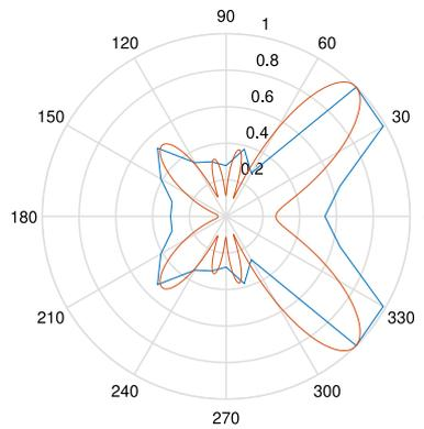
**Fig. 2:** Directivity characteristic at a frequency of 5 kHz. Comparison of calculation results (red) and experiment results (blue).
