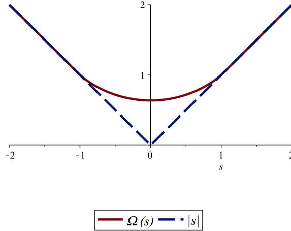
$$\Omega(s) = \begin{cases} (2/\pi)(s \arcsin s + \sqrt{1 - s^2}), & \text{for } |s| \leq 1 \\ |s|, & \text{for } |s| \geq 1 \end{cases}$$
